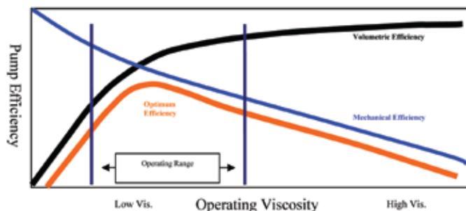
If a system's operating temperature could be maintained at exactly the same level throughout the operation cycles of the system, then the system could operate at peak efficiency.<sup>1</sup> Unfortunately, anything that influences operating temperature of the oil in the sump influences the systems' overall efficiency. Change in temperature and, consequently, viscosity is a double-edged sword. Operating temperature is influenced by many routine operating factors, including:
