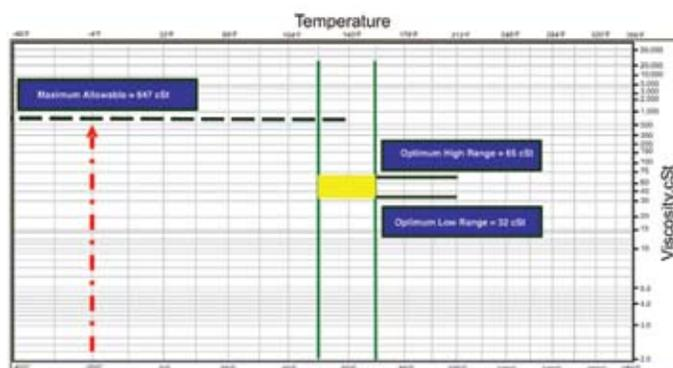
**Step 3.** Plot the optimum high, low and maximum viscosity for cold-start conditions on a temperature-viscosity chart (available from all oil company customer service departments). This step is shown in Figure 5. Determine the optimum working range on the viscosity reference chart. This is noted in yellow in the example. This represents the area that the best lubricant selection will occupy.
