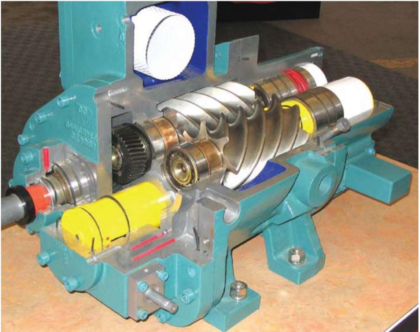
Figure 5 | Cutaway View of a Piston and Lube Rotor Set, including Timing Gear
