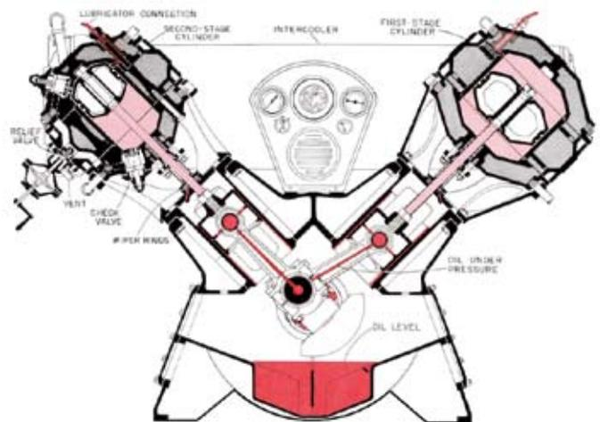
Figure 2 | V-Type Double-Acting, Two-Stage Compressor Showing Key Components (Courtesy of ExxonMobil Oil Corp.)
