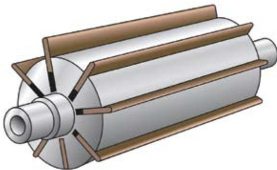
Figure 3(b) | The Position of Vane Placement Within a Rotor Under Operating Conditions
