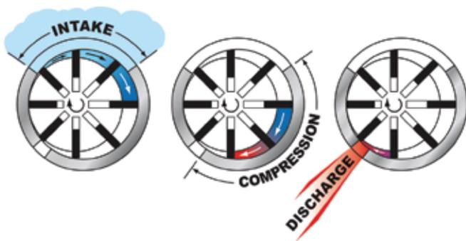
Figure 3(a) | Operation of a Vane Compressor Suction, Pressurization and Discharge Cycles
